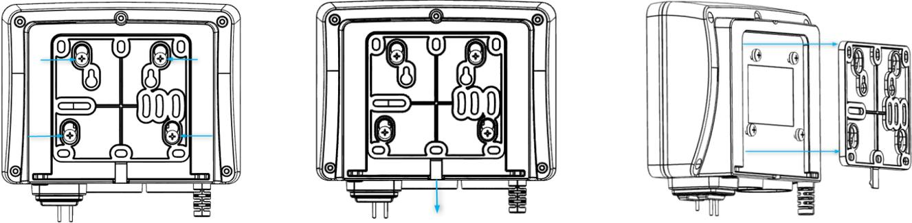
Ensure the tongue is facing down, mark four holes to mount the plate, and drill and screw to the wall. Ensure the plate is flat after tightening the screws so the DTAC may slide on and off easily. The mounting plate has multiple slots and holes allowing it to alternatively be mounted directly to screw holes from other legacy controllers.
