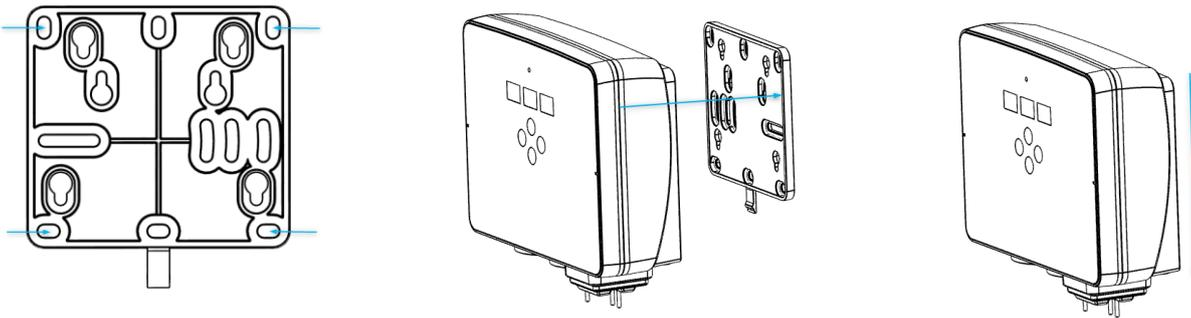
Align the DTAC housing and the mounting plate, then push the housing down to lock the unit on to the wall.
